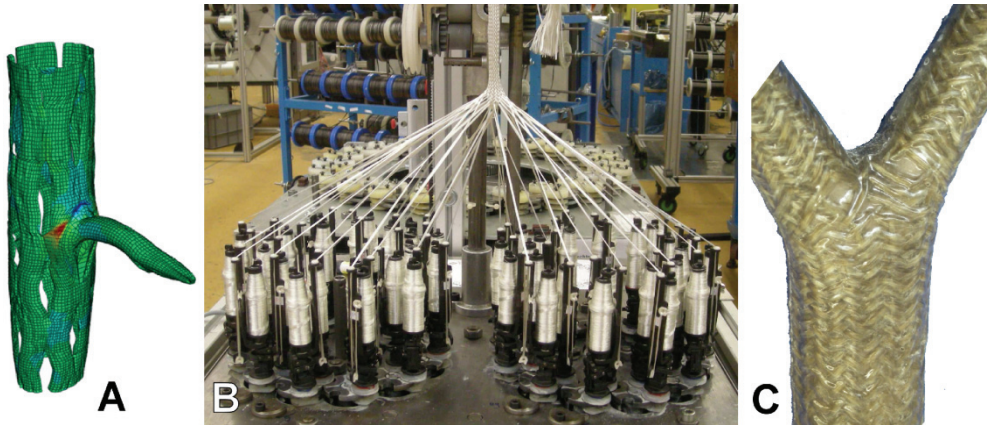
Fig. 28. (A) Simulated notch stresses in a stem-branch attachment region of a columnar cactus, (B) double braiding unit for producing branched braidings and (C) prototype of a braided Y-shaped preform. © (A) ILK Dresden, (B, C) ITV Denkerdorf.
