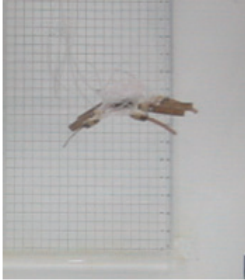
Fig. 20. Floating motion of the eight-legged microrobot
