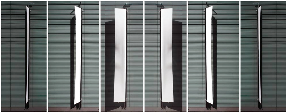
Fig. 12. Demonstrator for a façade shading system able to bend sideways up to an angle of 90° inspired by the kinetic system found in the flower of Strelitzia reginae . Torsional buckling and displacement of the lamina are induced by slightly bending the supporting rod. © itke University of Stuttgart.
