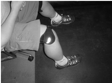
Fig. 6. Wearable and wireless accelerometer device mounted at lateral epicondyle adjacent to the knee joint
