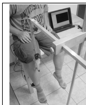
Fig. 2. Third generation wireless accelerometer reflex quantification device
