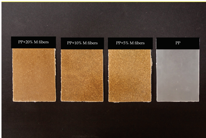
Fig. 4. Biodegradable flax composites made of polypropylene (PP) enriched with different content of bioplastic flax fibres (M plants). The control composite is made of polypropylene with no addition of flax fibres
