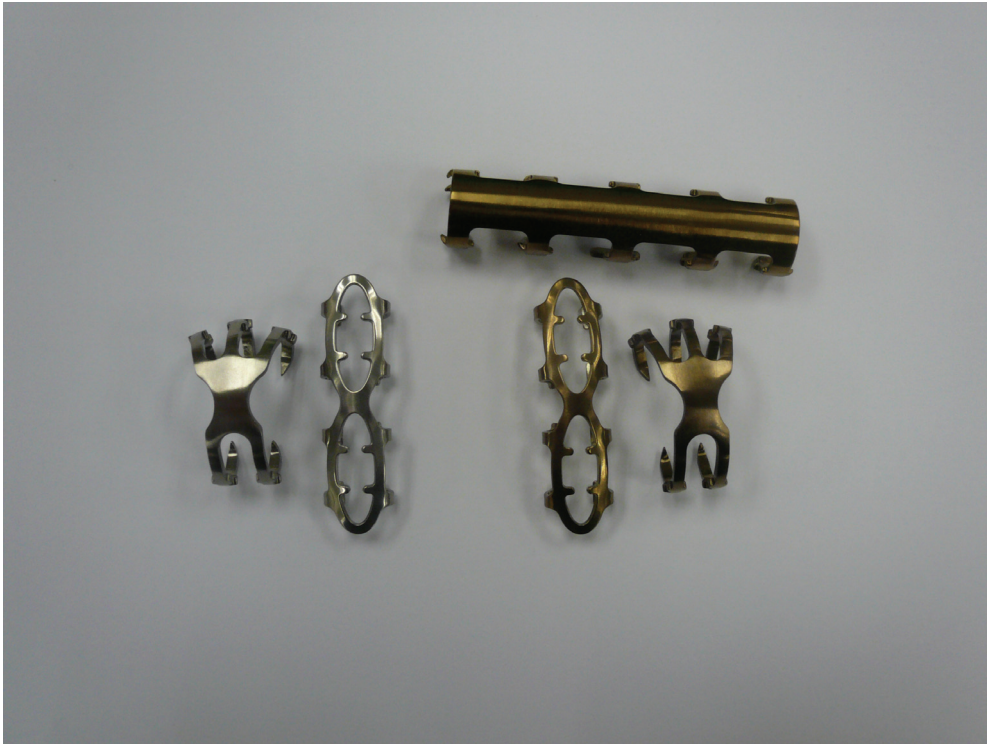
Fig. 6. Patellar concentrators and other bone concentrators with the left one showing two raw concentrators and the right one showing the three concentrators after the quasi DC-PIII treatment.
