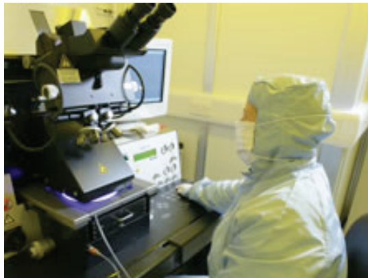
Fig. 3. The photolithographic patterning is done on a mask aligner where accurate exposure can be controlled. Image courtesy of the James Watt Nanofabrication Centre @ Glasgow
