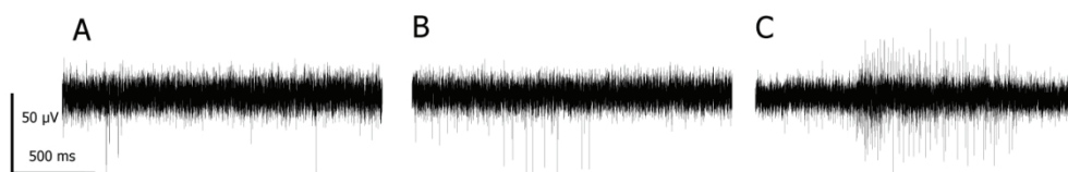
Fig. 2. Development of signalling in MEA. (A) First, after the neuronal cells have grown few days on MEA, first signals are detected. They are individual single spikes. (B) Then, about after 1-2 weeks of culturing spiking activity matures into training phase. There are several spikes organised together. (C) Finally, bursting activity occurs. Burst is a complex signal package that happens in several channels at the same time.
