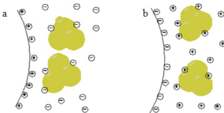
Fig. 1. a) Anionic (negatively charged) proteins exchange. b) Cationic (positively charged) proteins exchange.
