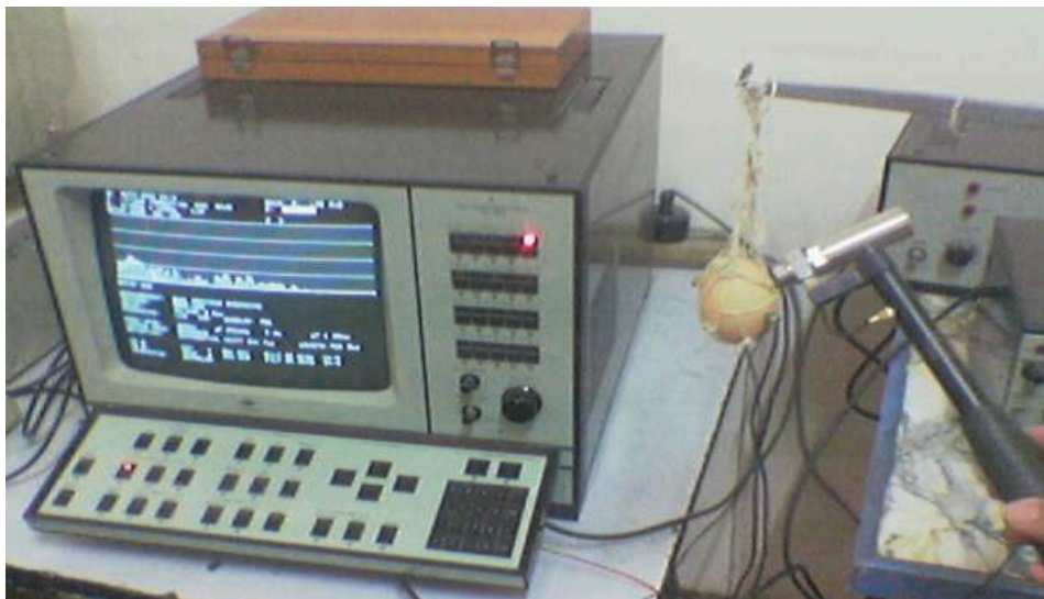
Fig. 3. (b) Free suspension for modal analysis.
