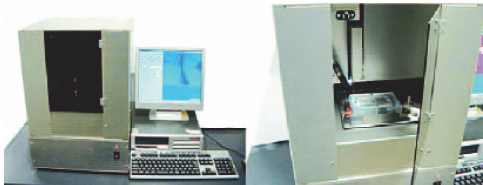
Fig. 2. Fully automated injection system for zebrafish
