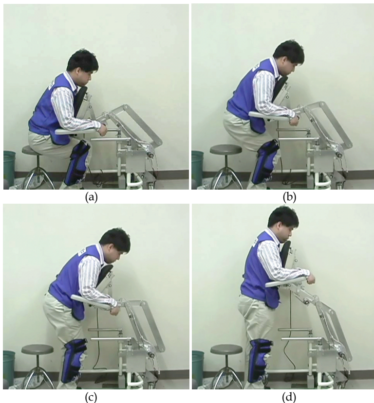
Fig. 15. Standing up motion with our system. (Our proposed scheme) The tester uses wearing equipment for the experience of the elderly (Takeda et al., 2001).
