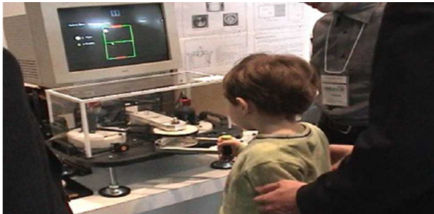
Fig. 32. Passive force display using ER brakes (PLEMO-P-Prototype).
