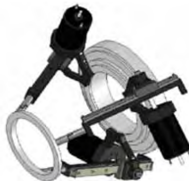
Fig 4. Wrist component of the MAHI arm exoskeleton employing electrical motors with a cable drive.
