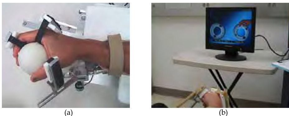
Fig. 3.6. HOWARD hand exoskeleton. (a)The exoskeleton allows practice of grasping with real objects; (b) practice of grasping in a VR environment. Adapted from (Cramer et al 2007).
