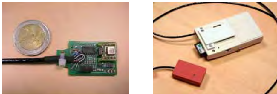
Fig. 3. CEA-LETI attitude sensor and its acquisition system. Left: Sensor size. Board is then embedded in a silicon-like material. Right: Final view of the sensor, with its datalogger.
