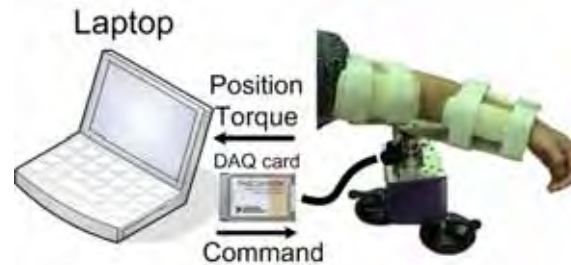
Fig. 2. Control diagram of the limb-stretching device: The device was controlled by a laptop for portability.
