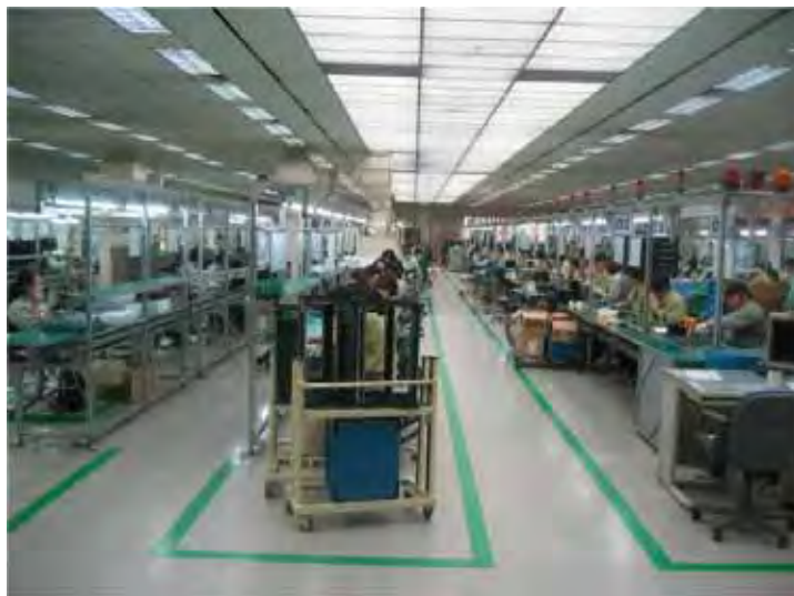
Fig. 7. Whole view of general environment of manufacturing factory. Safety lines are painted around work tables.
