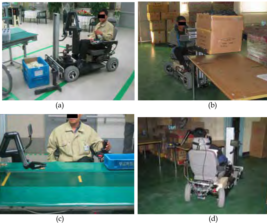
Fig. 14. User trials for Work Assistive Mobile Robot System Type I; (a) Moving objects - lifting up, (b) Moving objects - lowering, (c) Working at a desk, (d) Moving around.
