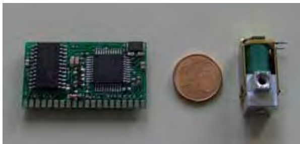
Fig. 4. Electric valve and control unit.
