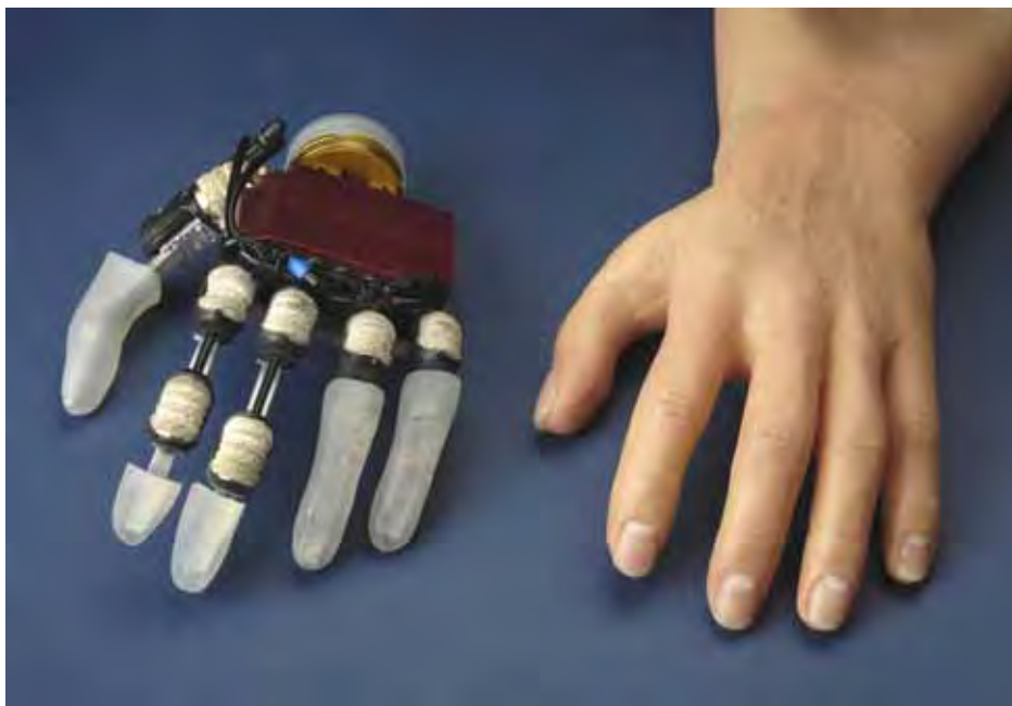
Fig. 19. A cosmetic glove made of silicone rubber covers the mechanics of the multifunctional prosthesis [Schulz 2005]. The thumb can be moved in a plane transverse to the index and middle finger.
