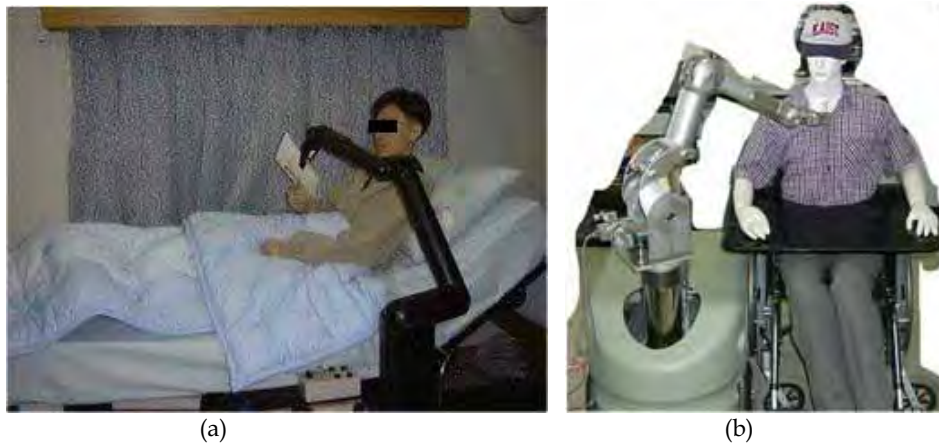
Fig. 1. Examples of robots for daily activities of the disabled; (a) Intelligent bed-robot system, (b) KARES II.
