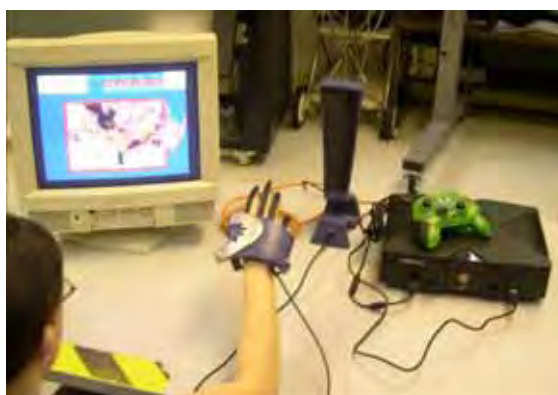
Fig. 3.5. Overall view of the experimental low-cost finger training system. Adapted from (Morrow et al., 2006).
