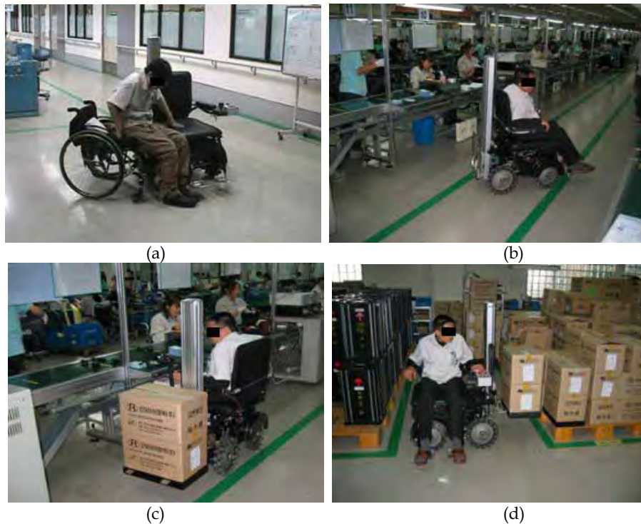
Fig. 20. User trials for Work Assistive Mobile Robot System Type II; (a) Transferring boxes, (b) Moving around, (c) Working at a desk, (d) Moving boxes.
