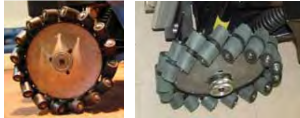
Fig. 15. Mecanum wheel for omni-directional movement.
