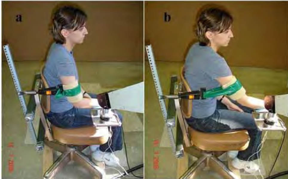
Fig. 5a. Initially No Resistance is Applied to the Participant's Upper Arm, Fig. 5b. Resistance is Applied to the Participant's Upper Arm in the Direction of Motion as the Task Begins.
