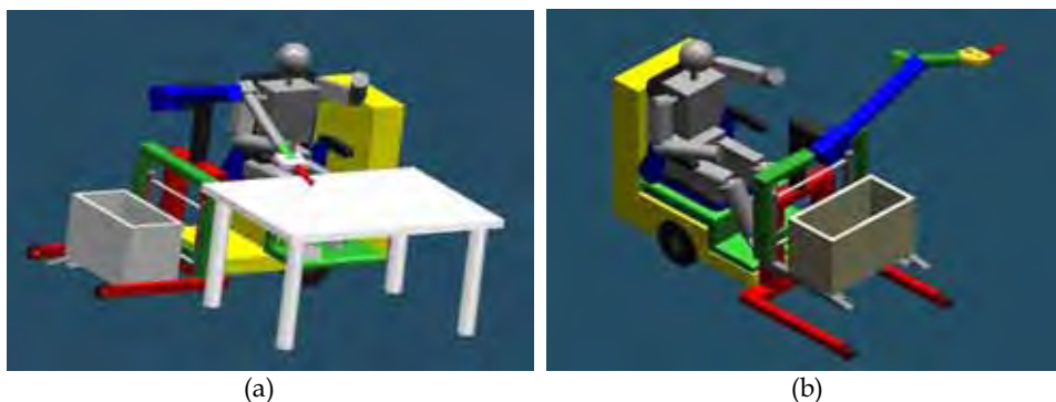
Fig. 11. Basic concept of work assistive mobile robot system type I; (a) assisting table tasks, (b) moving objects.
