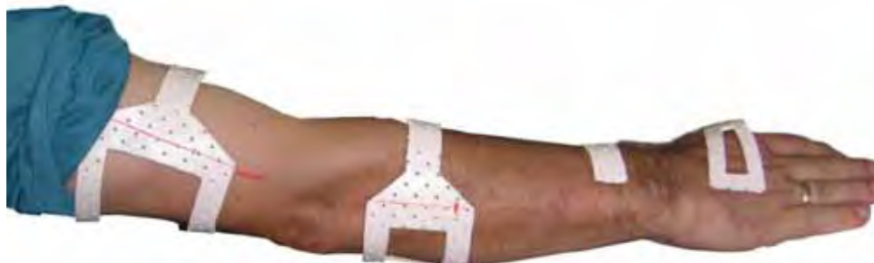
Fig. 1. Illustration of the WOTAS supports on a patient's arm. The supports are manufactured in thermoplastic to best adapt to the morphology of each user's arm.
