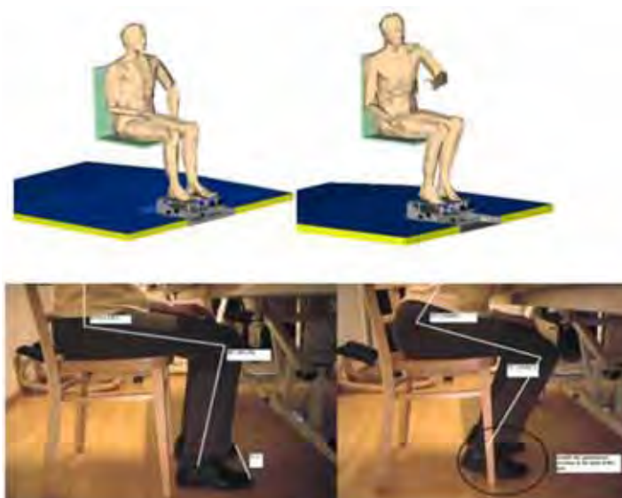
Fig. 1. CAD models used in the ergonomic study (top) and the two selected postures for the lower extremities and the feet (bottom).
