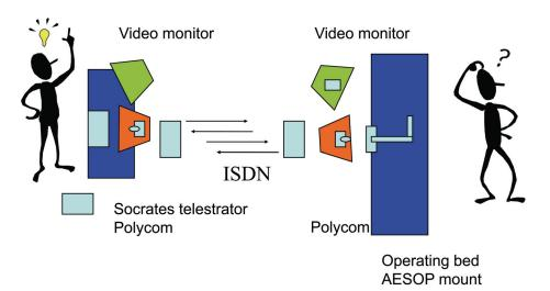
Fig. 1. Telementoring set-up. The set up in our telementoring procedures involved 4 ISDN lines as well as audiovisual Polycoms, and video screen telestrator. The AESOP laparoscope holding robot was used during early, but not later clinical use. The mentor is pictured on the left while the trainee along-side the OR table is pictured on the right hand side.
