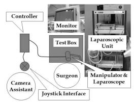
Fig. 11. Installation of devices in *in-vitro* experiment
