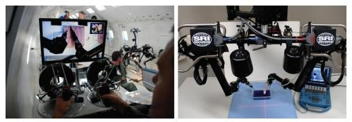
Fig. 7. The M7 on board of a NASA parabolic flight, and the robot performing autonomous ultrasound-guided tissue biopsy. (Photo: NASA, SRI)
