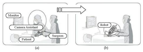
Fig. 1. Endoscopic surgery (a) A human camera assistant operates the endoscope. (b) An endoscope robot operates the endoscope.
