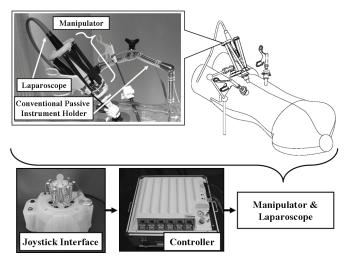
Fig. 5. System configuration
