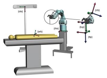
Fig. 2. Coordinate systems – {ots} localizer (<u>optical tracking system</u>), {arb} patient (<u>a</u>im <u>r</u>eference <u>body</u>), {rrb} (<u>robot r</u>eference <u>body</u>) {rbs} <u>robot base</u>, {tcp} robot wrist (<u>tool center point</u>), {ttp} <u>tool tip</u>
