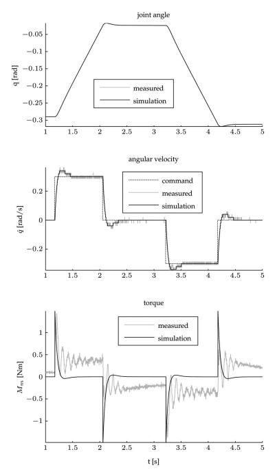
Fig. 5. Simulation results using the identified servo model compared to real measurements (dataset for identification), exemplary for the first shoulder joint (*S*1)
