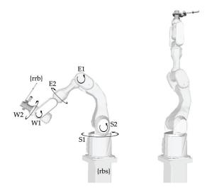
Fig. 7. Differing poses for robot dynamics identification (left) and exemplary verification (right)
