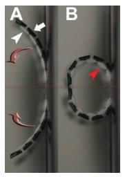
Fig. 9. The Microhand forceps is a four-fingered Microhand articulated by six silicone phalanges (A, white arrow) and joined by inflatable balloons (A, arrow heads). When balloons are inflated (B, red arrow head), fingers are incurved (A, red arrows and B) and face themselves along the central axis (red line). From Hubschman, J. P., J. L. Bourges, et al. (2009). "The Microhand': a new concept of micro-forceps for ocular robotic surgery." Eye.
