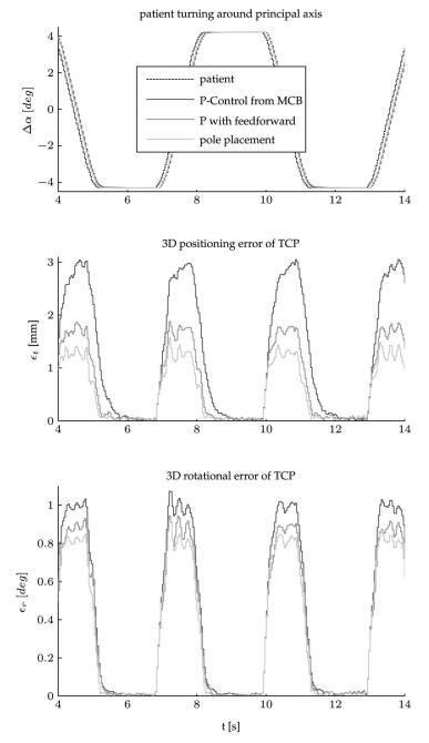
Fig. 10. Comparison of three different control strategies - 1. original proportional controller, 2. proportional with feedforward, 3. pole placement controller
