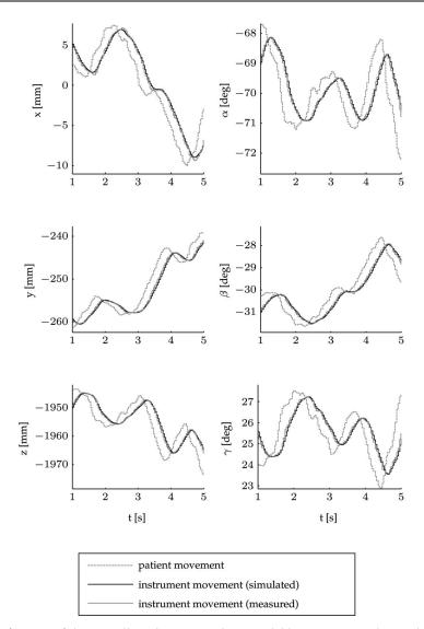
Fig. 8. Verification of the overall tracking procedure model by comparing the model output signals to real measurements (cartesian time trajectories of robot wrist pose)
