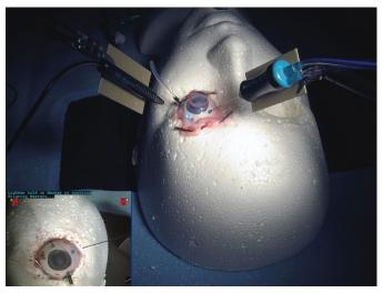
Fig. 8. Insertion of the modified 25-gauge vitreous cutter and endo illuminator with the robotic arms. Left corner - high magnification view through the robotic endoscope.
