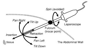
Fig. 4. Movement of endoscope: Since the endoscope is limited due to the insertion site, the endoscope has four degrees of freedom.
