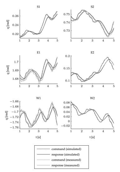
Fig. 9. Verification of the overall tracking procedure model by comparing the model output signals to real measurements (time trajectories of robot joint angles)
