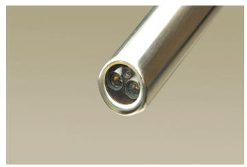
Fig. 2. Endoscope which has two lenses
