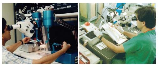
Fig. 3. The RAMS robot developed at NASA JPL in laboratory trials and in-vivo animal tests in 1998. (Photo: NASA)
