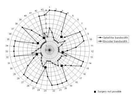
Fig. 4. Satellite and encoder bandwidths were sequentially decreased to identify a minimum level for telesurgery. The bandwidth 'pipe' is shown as concentric circles (9–0 Mb/s). Changes in bandwidth combinations using 7 pigs are seen radially in the 43 spokes. ■, satellite bandwidths at which surgery was no longer possible (approximately 4 Mb/s)
