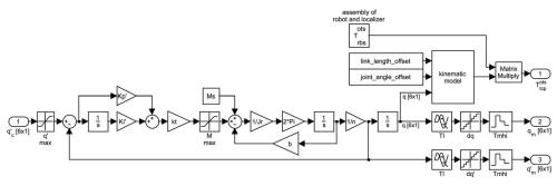
Fig. 4. Robot model - kinematics and joint servo dynamics
