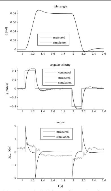
Fig. 6. Simulation results using the identified servo model compared to real measurements for the first shoulder joint (*S*1) in one exemplary scenario different to the identification scenario
