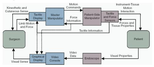
Fig. 1. Integration of different modality feedback information to the concept of telesurgery. Interaction is only possible through a system of sensors and human-machine interfaces. Modified from (Hager et al., 2008).
