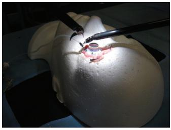
Fig. 7. The *da Vinci* surgical system was used to insert 3 trans-scleral cannulas which is necessaary for minimally invasive vitrectomy surgery. In addition to axial motion, the wrist-like tips of the robotic instruments have roll, pitch, yaw and grip to facilitate delicate manipulations.
