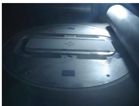
Fig. 1. Selective laser sintering of PLLA/CHAp powder in progress.
