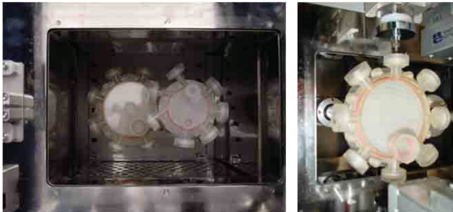
Fig. 13. Two vessels in the CO 2 incubator in the automatic RWV culture system (left) and the vessel out of the incubator with two attached syringes (right)
