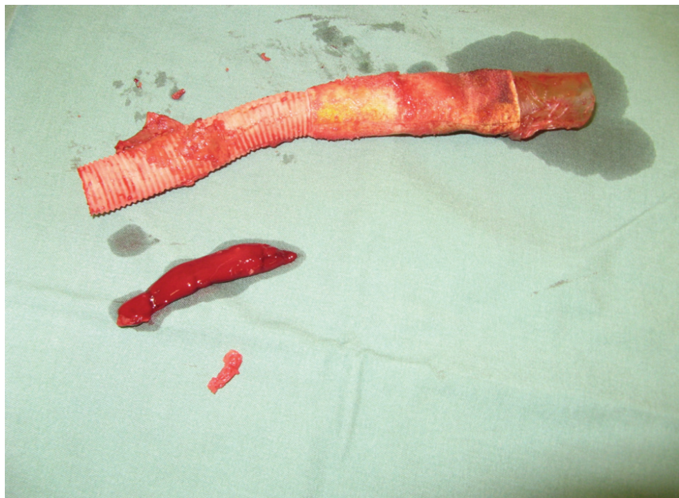
Fig. 8. Thrombus found within a VAD cannulae following an alarm for low VAD flows
